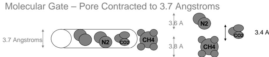
*Figure 4 - Schematic of the Molecular Gate Adsorbent Separation*
