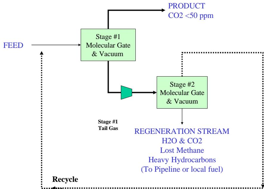
Figure 7 - Two Stage Processing Schematic #2
