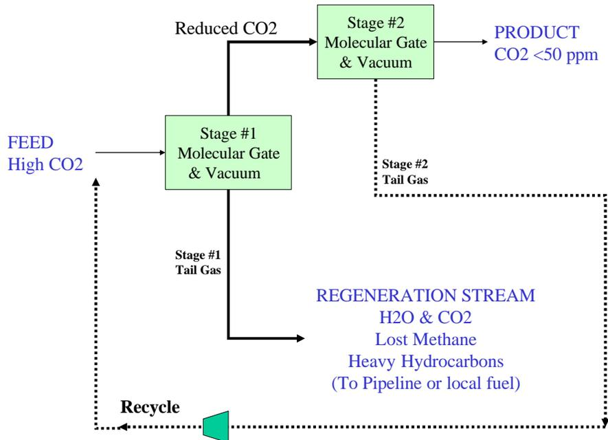
Figure 6 - Two Stage Processing Schematic #1
