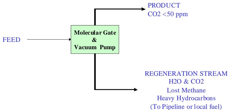
Figure 5 - Typical Single Stage Molecular Gate Processing
