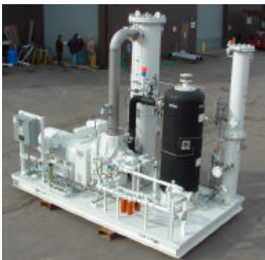
A Guild packaged biogas feed compressor
