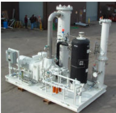
*A Guild packaged biogas feed compressor*
